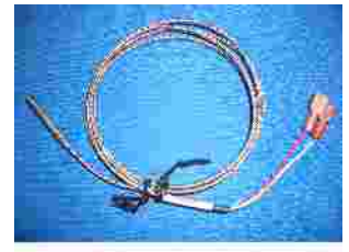
Thermocouple - Dig Oven
